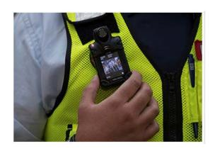
Small and wearable electronic devices used in workplaces (e.g., body cameras) rely on a power source that stores a high amount of energy in a small space (i.e., high energy density). Lithium cells provide sustained power and often have the capability to recharge. When designed, manufactured, and used properly, lithium batteries are a
